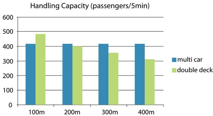
Graph 3: Comparison of multicar vs. double deck depending on travel height: handling capacity. Source: ThyssenKrupp
