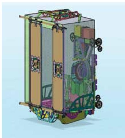
Opposite: A circulating rope-less elevator system called MULTI. Source: ThyssenKrupp
