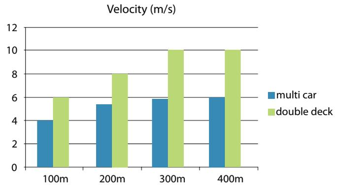
Graph 4: Comparison of multicar vs. double deck depending on travel height: velocity. Source: ThyssenKrupp
