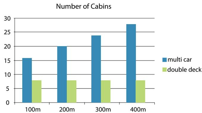
Graph 5: Comparison of multicar vs. double deck depending on travel height: number of cabins. Source: ThyssenKrupp
