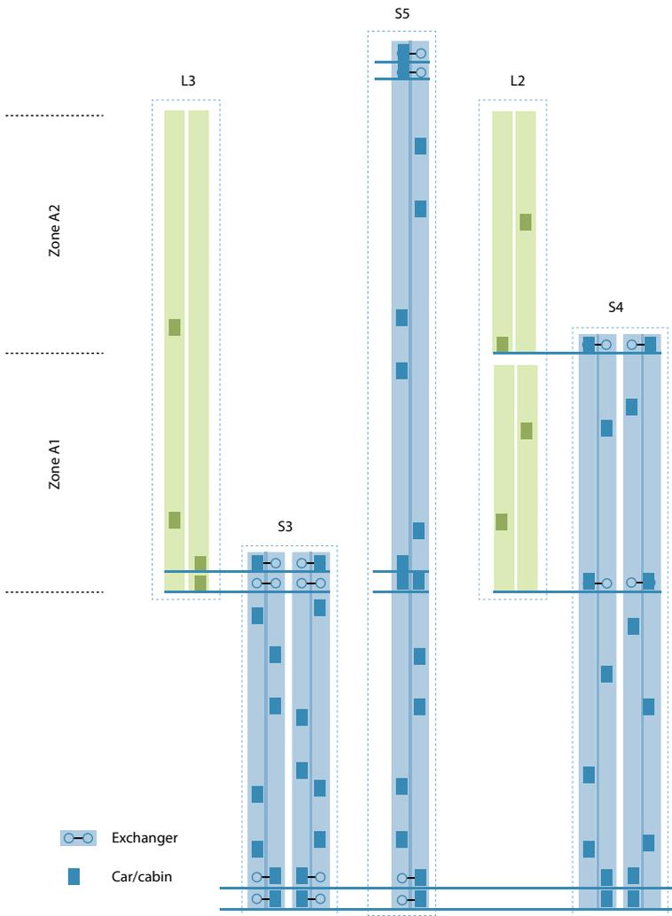
Left: Options of simplified traffic concepts including a circulation multicar system as a shuttle with a double ground lobby. Source: ThyssenKrupp
