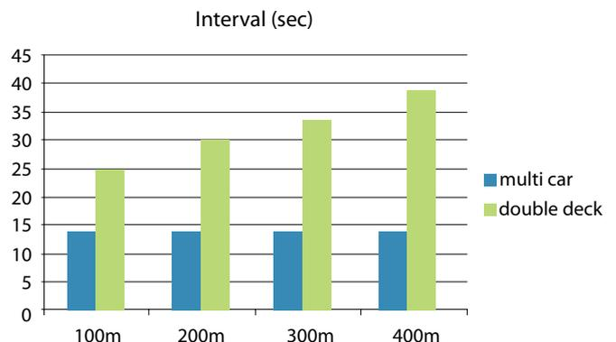
Graph 6: Comparison of multicar vs. double deck depending on travel height: interval. Source: ThyssenKrupp
