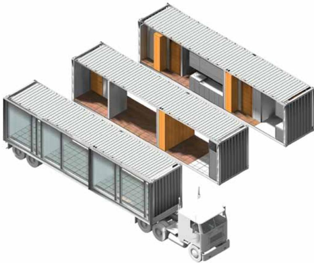
with the eight steel corner nodes which enable automated intermodal handling. We'll call that new type of building module a Volumetric Unit of Construction, or VUC, to clearly distinguish it from a shipping container.
