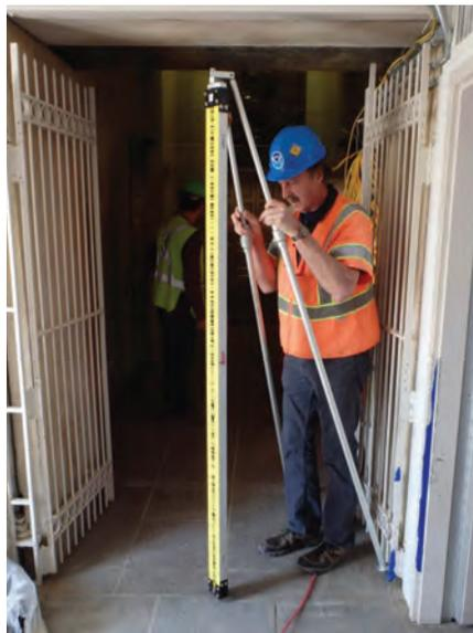
Figure 2. Height is measured from the level of the lowest, significant, open-air, pedestrian entrance to the architectural top of the structure (CTBUH criteria).
