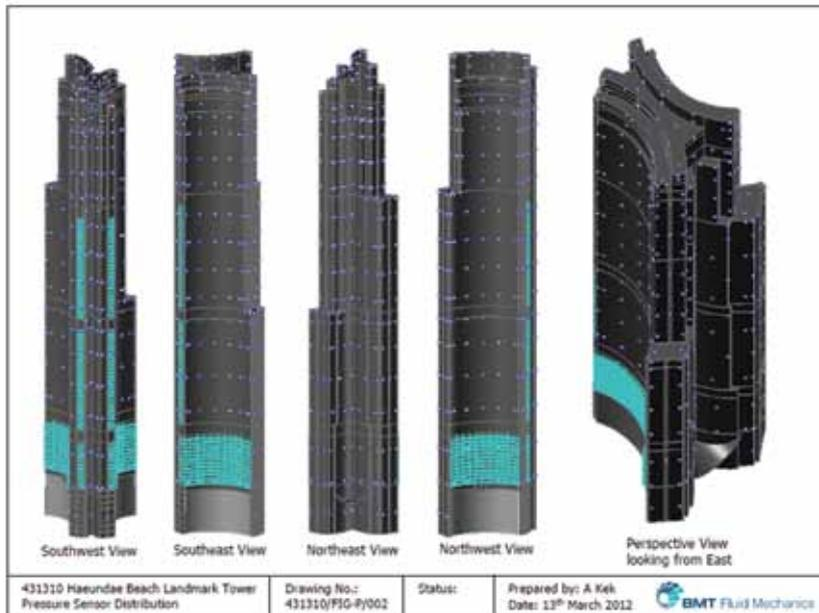
Left: The cladding maximum (positive) pressure and minimum (negative) pressure in elevation for each tower is general 4-6 KPa. But worst point from graphical presentations of rationalized block diagram is closed to -8~-9 Kpa.
