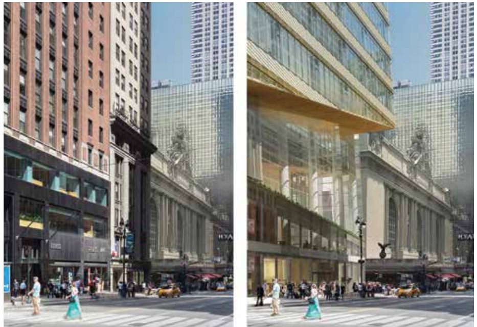
Figure 8. Existing (left) Proposed (right), currently, buildings on site obstruct a view to Grand Central Terminal. One Vanderbilt reveals the Grand Central cornice and corner for the first time in over 100 years. This feat is achieved through a sloped massing, angled cuts at the base, and a highly transparent glass atrium space (Source: Kohn Pedersen Fox Associates)
