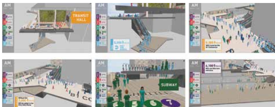
Figure 7. Projected Transit with East Side Access, East Side Access will bring an estimated 94,000 daily riders to the Grand Central District. As part of the ULUPR application, transit projections were simulated and explained in an animated video (Source: Kohn Pedersen Fox Associates)
