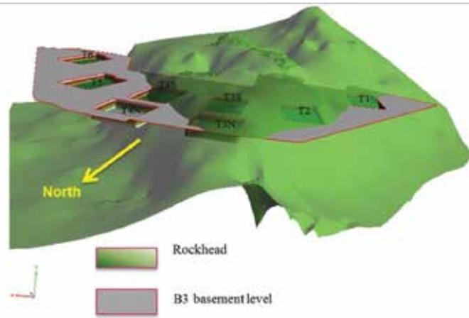
Figure 14. Rockhead contour (Source: Arup)
