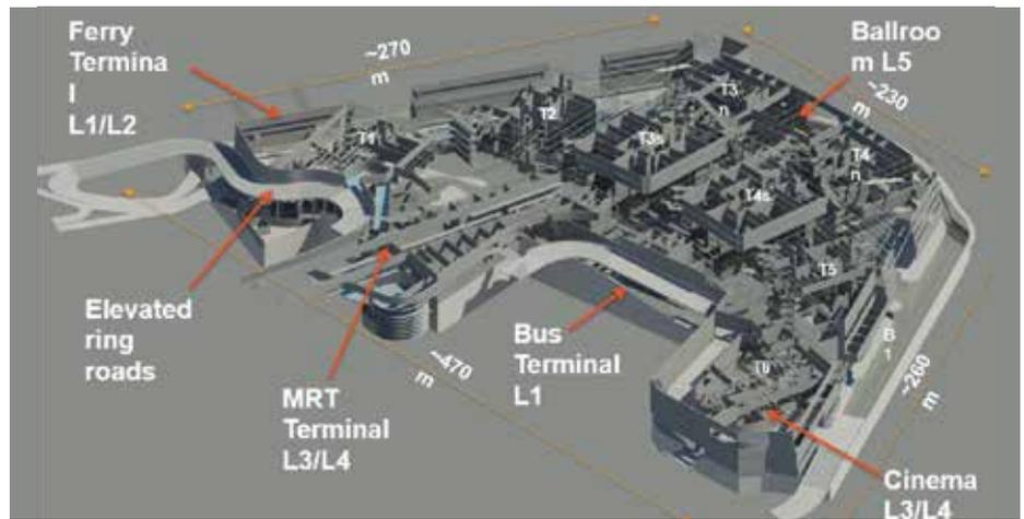
Figure 11. Revit model extract of the podium and major program zones (Source: Arup)
