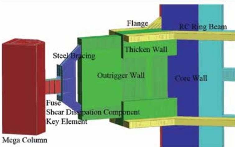
Figure 8. Hybrid outrigger system (Source: Arup)
