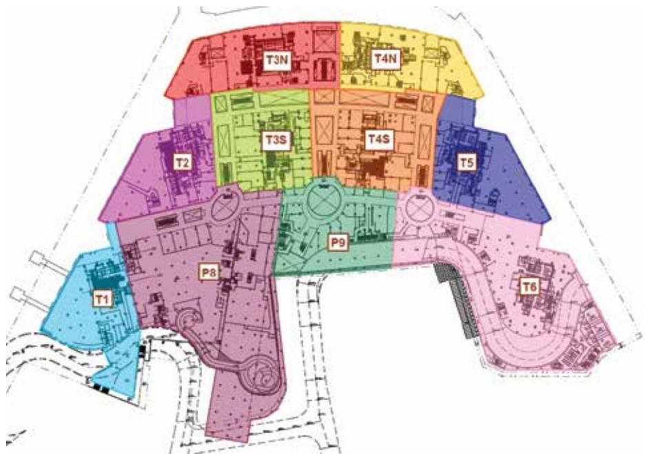
Figure 12. Movement joints in the podium structure (Source: Arup)
