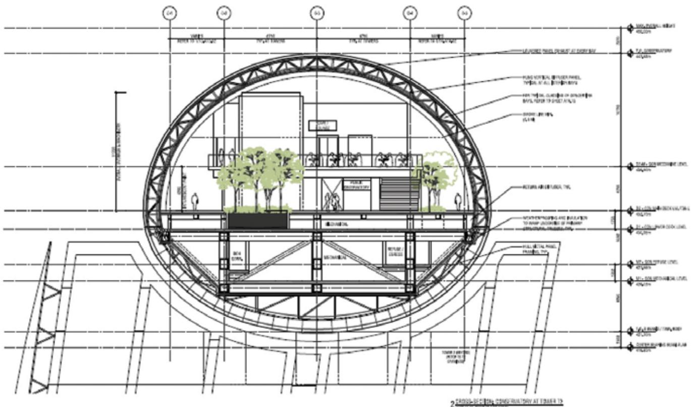
Figure 7. Section showing light-weight trussed enclosure to conservatory (Source: Arup, courtesy of Moshie Safdie Architects)
