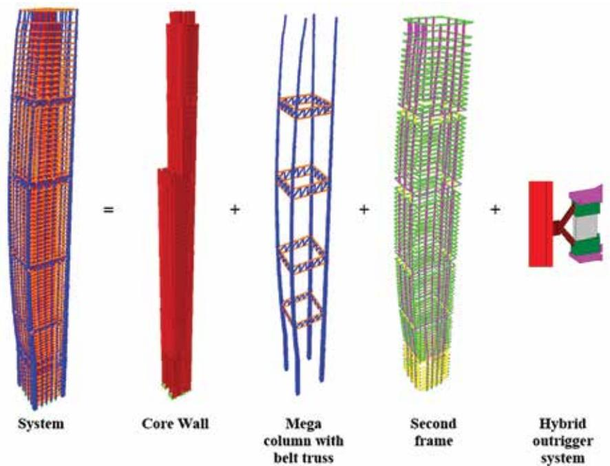
Figure 3. North towers structural stability system (Source: Arup)
