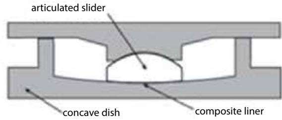
Figure 6. Friction pendulum bearing (Source: Arup, courtesy of Maurer Soehne GmbH & Co)
