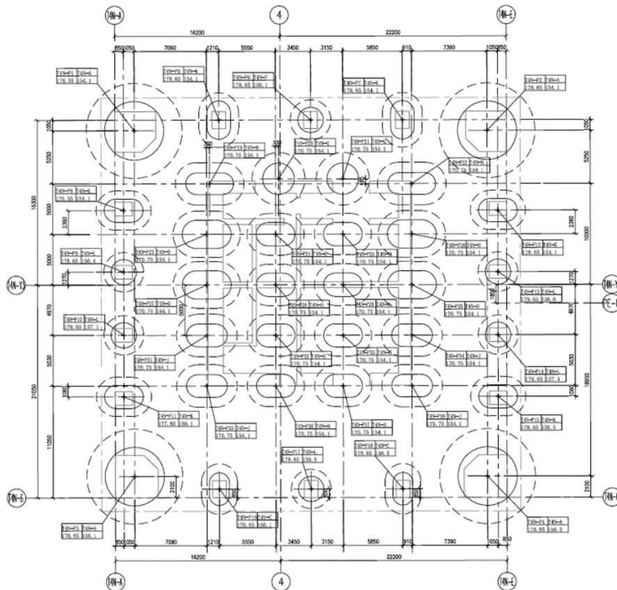
Figure 15. Foundation plan of the north tower (Source: Arup)
