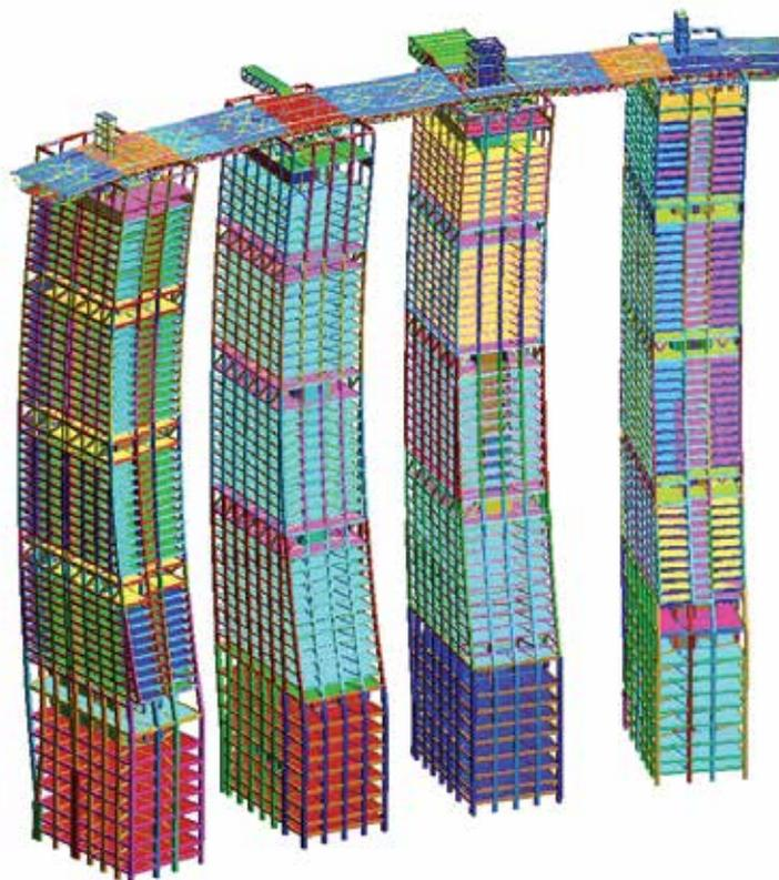
Figure 5. LS-Dyna model for non-linear time-history analyses in conservatory articulation (Source: Arup)
