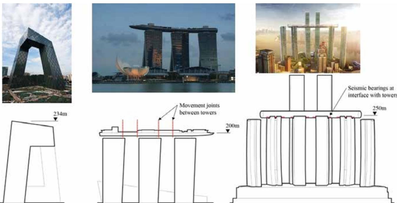
Figure 4. Comparison of long span and cantilevered horizontal structures at height (Source: Arup)
