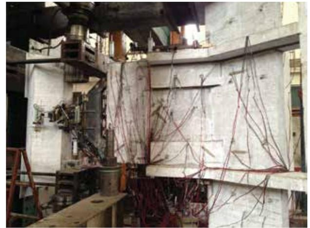
Figure 9. Prototype testing of the hybrid outrigger system (Source: Arup)
