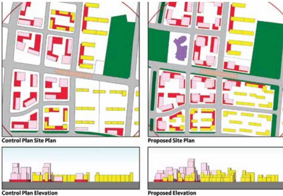
Figure 8. Focusing development at a transit node intensifies development at the transit opportunity and allows for the evolution of a skyline. INCENTIVISED DEVELOPMENT CONTROLS. (Source: Gensler)
