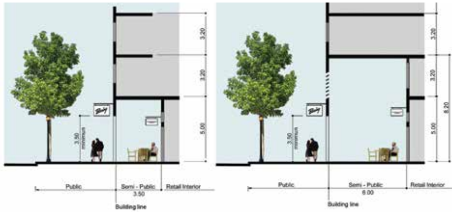
Figure 11. A variety of ratios were developed for the Master Plan for Bandar Seri Begawan, the capital of Brunei, which is near the equator on the island of Borneo. The Master Plan put in place regulations that made building arcades mandatory for all new construction in the CBD. ARCADE DESIGN GUIDELINES. (Source: The Office of Tom Ford/HOK Asia Pacific)
