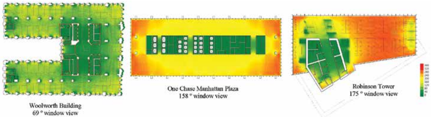
Figure 5. Window Access: A comparative analysis of window access across buildings built over the last 100 years. The amount of window access increases dramatically with each new era's exemplar. Workstations in Robinson Tower averages a 265° window view from workstations (Source: NBBJ)
