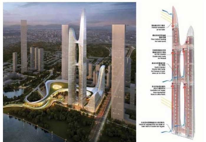
Figure 3. Rendering of Liansheng Financial Tower with ventilation diagram (Source: SOM)
