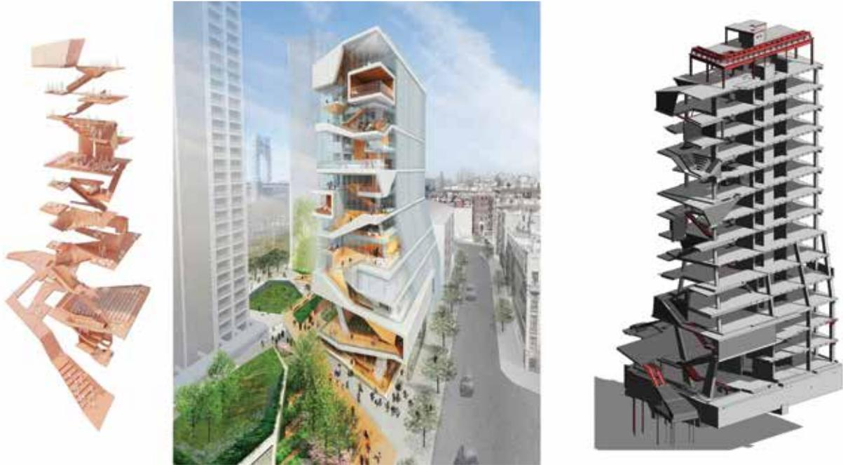
Figure 3. “Wood-lined living room” of the Cascade and corresponding structural challenges of varied spatial planning. (Source: (left image) Diller Scofidio + Renfro / (right image) Leslie E. Robertson Associates)
