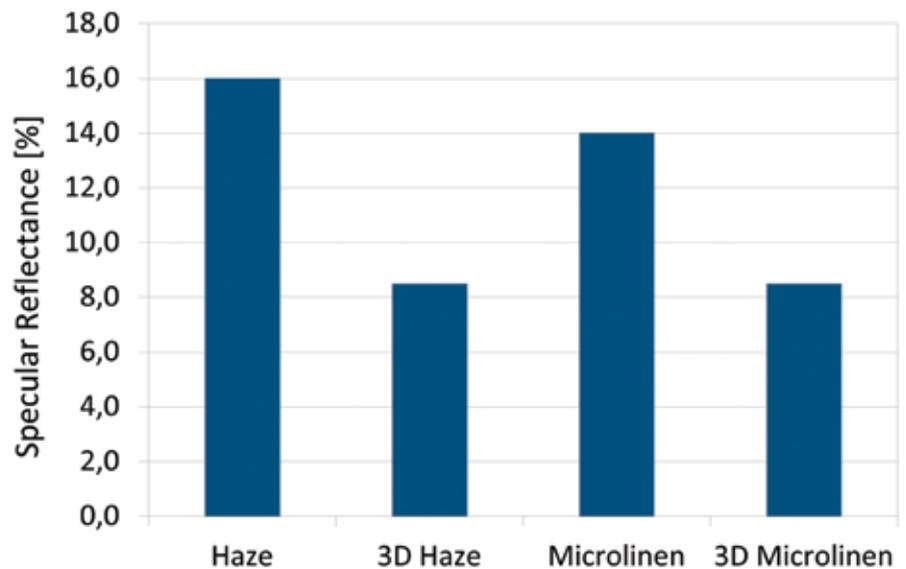
Figure 4. Decrease of specular reflectance due to additional rolling of coarse pattern (Source: Outokumpu)
