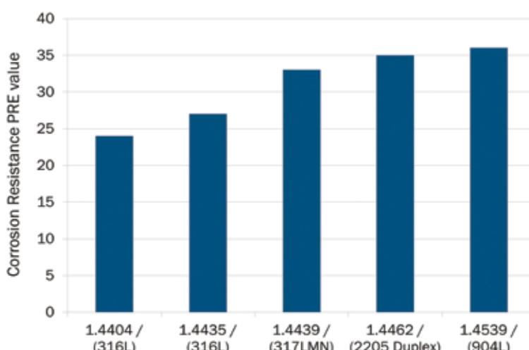
Figure 7. Comparison of the PRE values for highly corrosion-resistant austenitic and Duplex grades (Source: Outokumpu)
