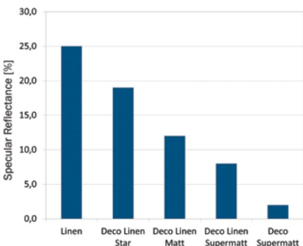
Figure 6. Comparison of specular reflectance for the newly developed Linen versions and Deco Supermatt (Source: Outokumpu)
