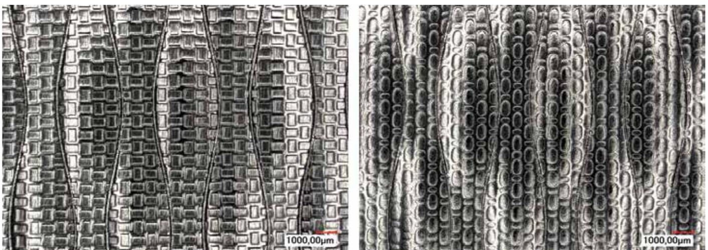
Figure 5. Microscopic images of 3D Haze (left) and 3D Microlinen (right) (Source: Outokumpu)
