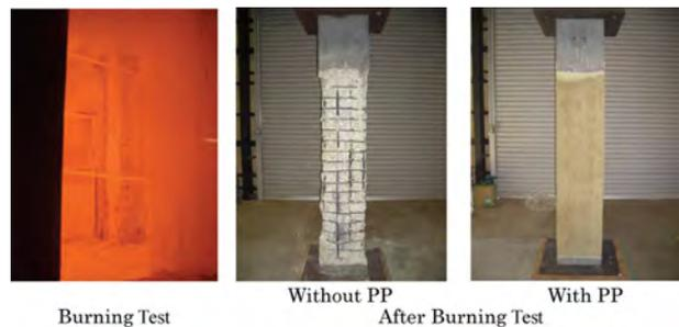
Figure 16. Fire Resistance Experiment.
