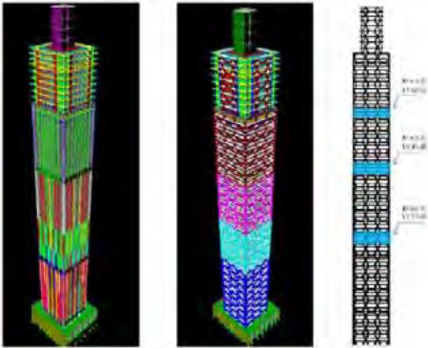
Figure 8. 3D Analysis model of the existing and HexaGrid towers, elevation indicating braced levels to HexaGrid (Source: Dr. Peyman A. Nejad)
