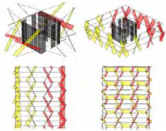
Figure 11. Axial force diagrams from lateral wind loading (Source: Dr. Peyman A. Nejad)
