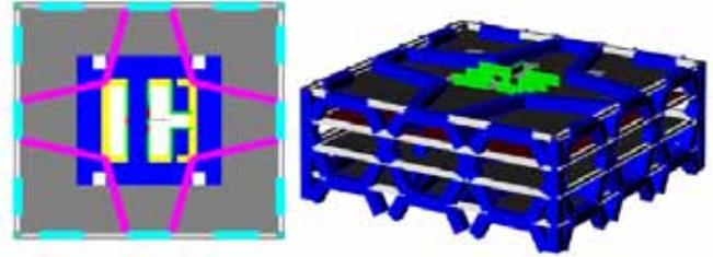
Figure 9. 3D and plan indicating braced levels (Source: Dr. Peyman A. Nejad)
