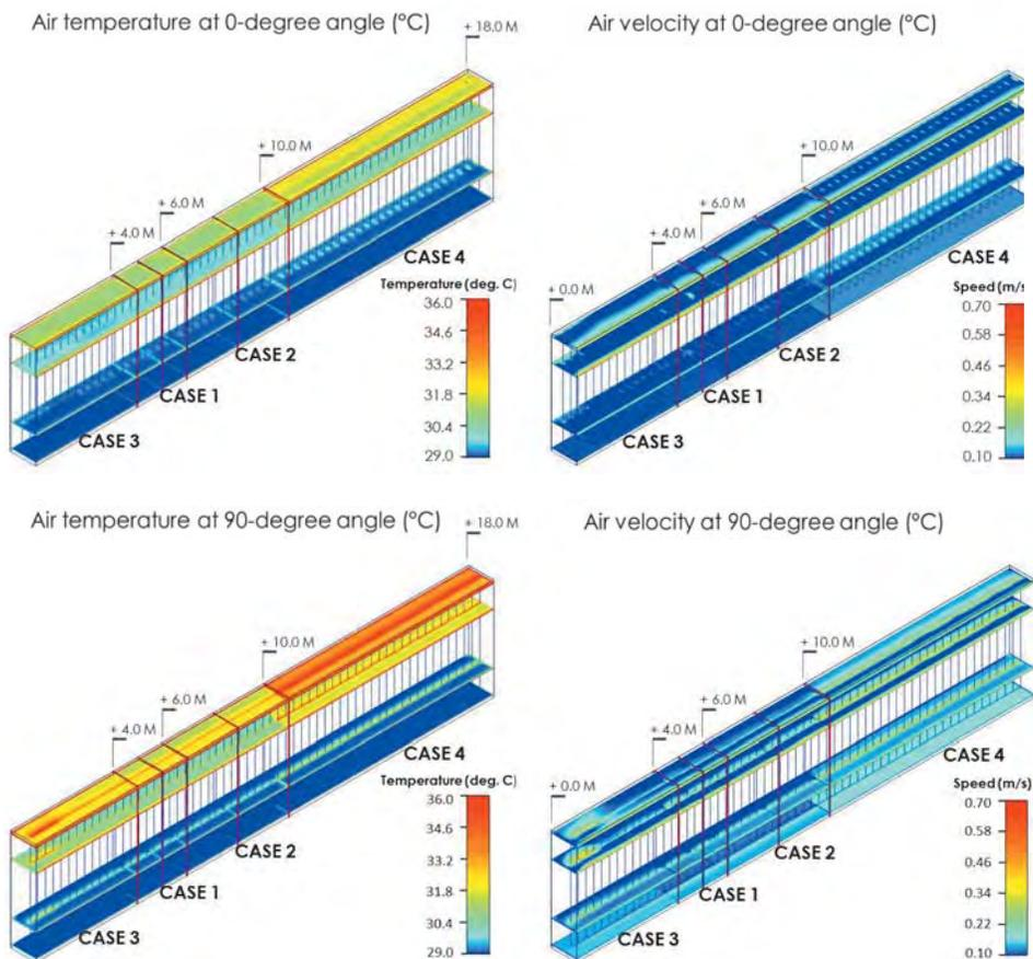
Figure 5. Air temperature and air velocity at 0- and 90-degree angles.
