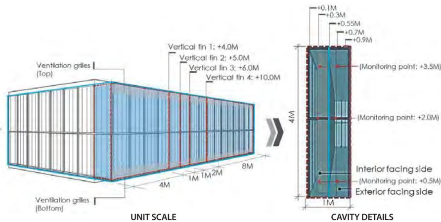
Figure 4. Unit scale and air cavity details for CFD simulation.
