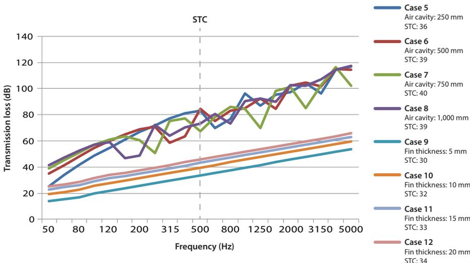
Figure 7. STC and STL by DSF air cavity depth and glass fin thickness.
