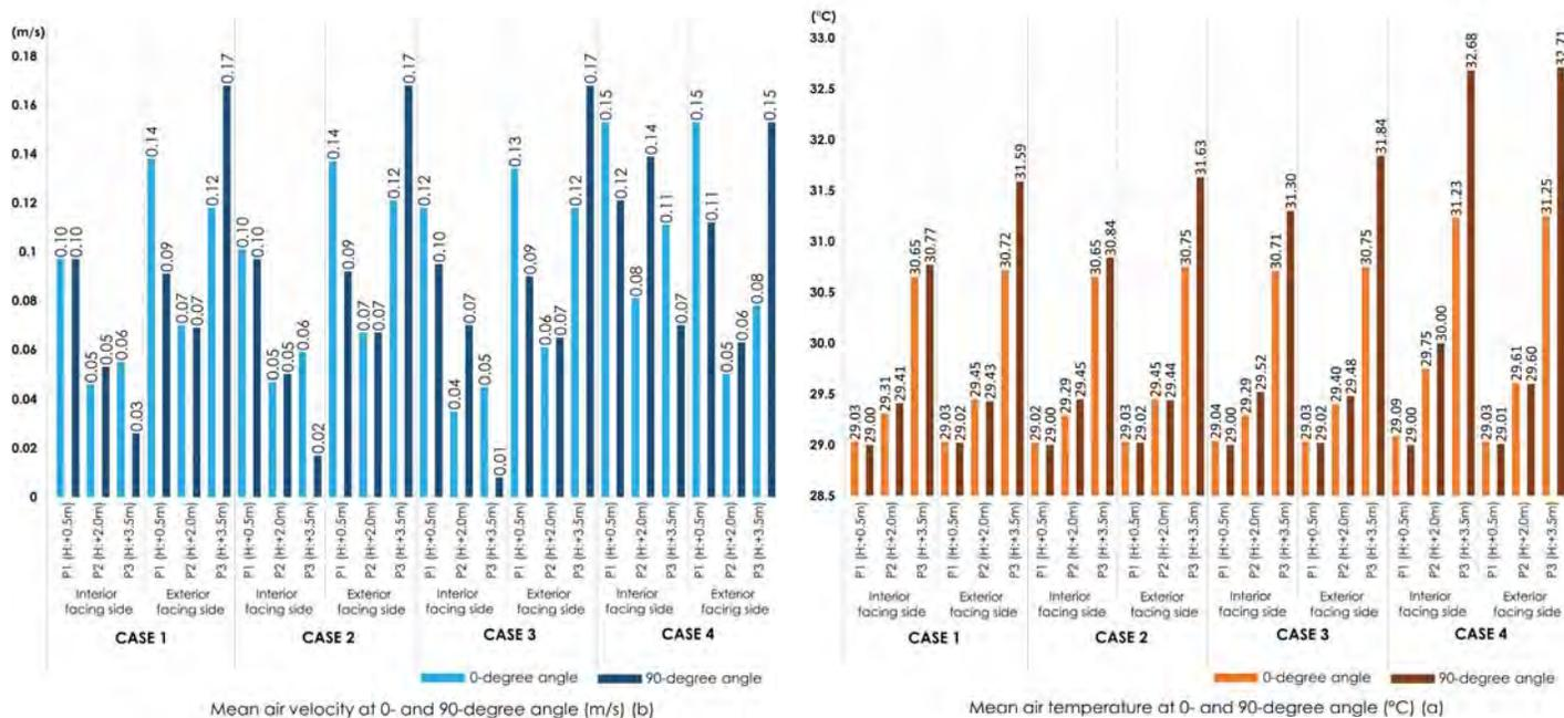
Figure 6. Mean air temperature and mean air velocity at 0- and 90-degree angle.
