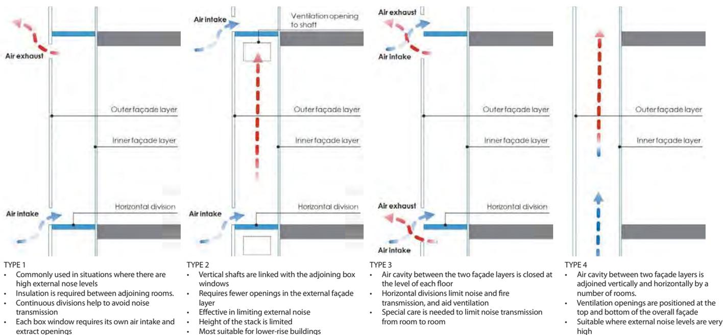
Figure 3. Airflow diagrams based on types of DSF air cavity design. Source: Oesterle et al., 2001.
