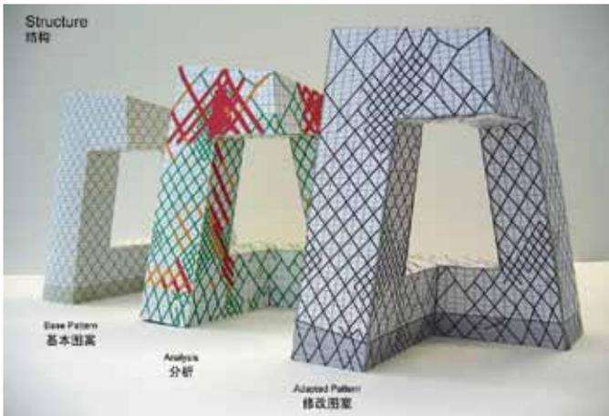
Figure 6: CCTV diagrid tube system with bracing pattern expressing structural forces. © Arup
