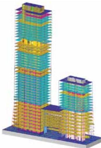
Figure 3: LS-Dyna Analysis Model of the Shenzhen Energy Headquarters Building. © Arup
