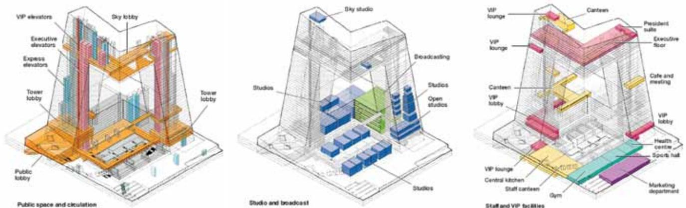
Figure 5: Functions and layout within the CCTV building. © OMA
