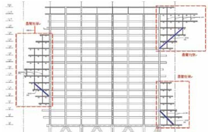
Figure 7: Shenzhen Energy Building – structural steel use restricted to the cantilevering blocks (South Tower wing elevation). © Arup
