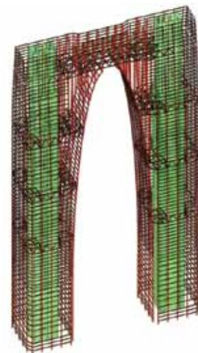
Figure 4: Suzhou "Gate to the East" - structural model for lateral stability analysis. © Arup
