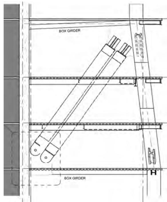
**Figure 4.** Bottom outrigger extending through three stories.
