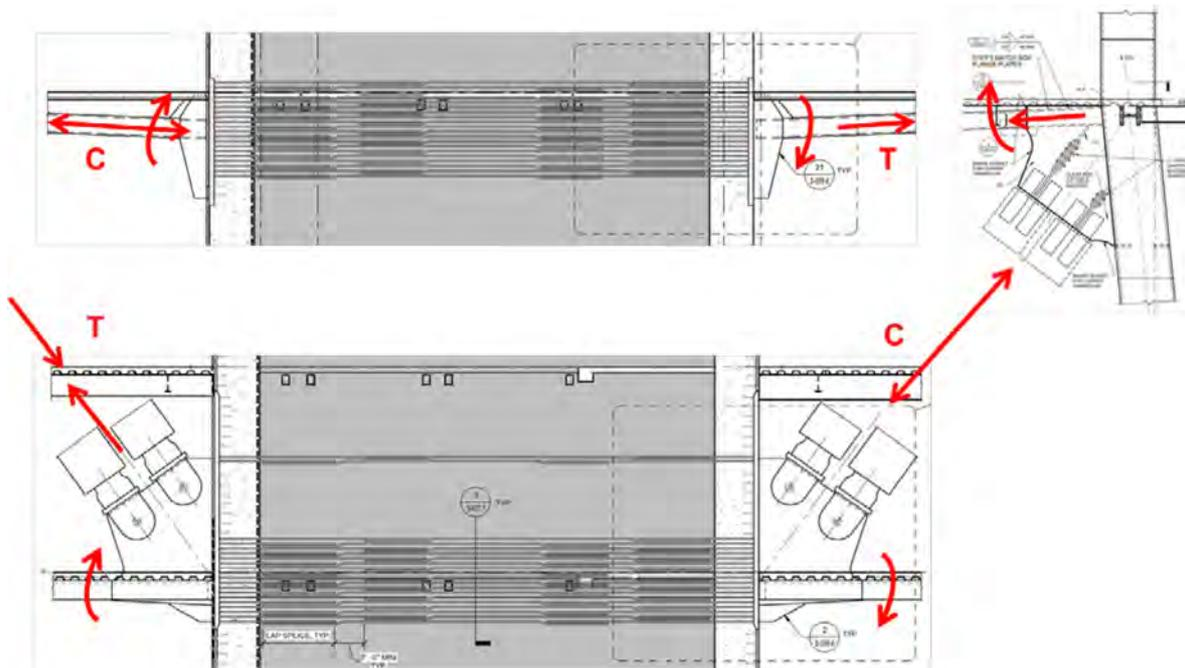
**Figure 15.** Simultaneous forces acting on bottom outrigger connections.
