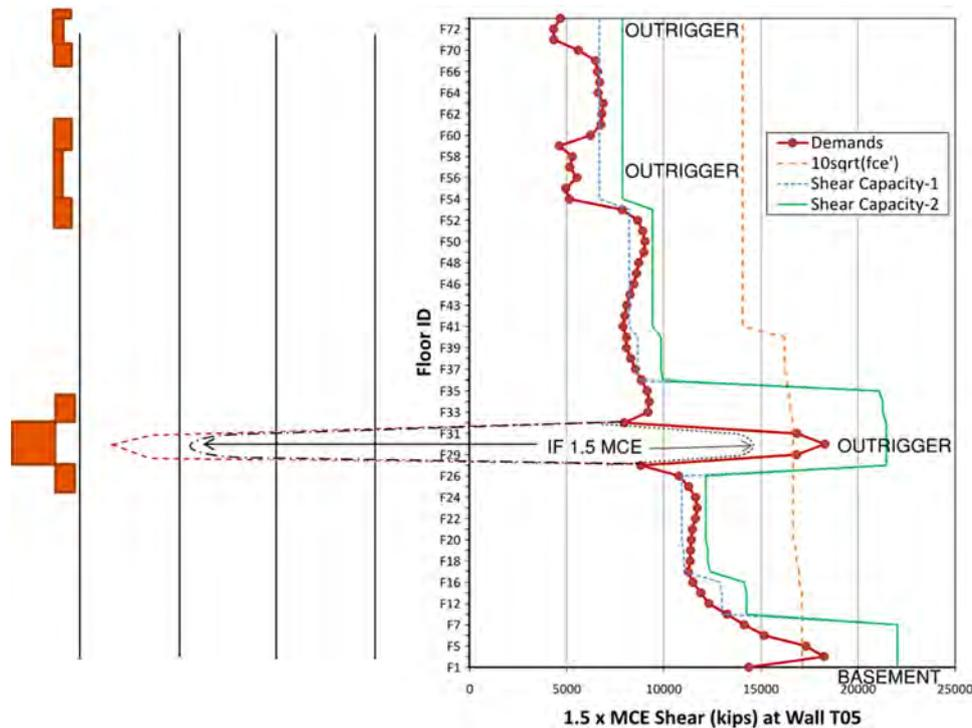
**Figure 14.** Wall shears at 1.5×MCE show ‘panel zone’ effects from outrigger force couples, reducing or even reversing wall shears as indicated by the core shear diagrams at left. Curves to left reflect reversal seen under static loading (solid curve to right shows ‘directionless’ results from dynamic analyses). Shear under mean of 1.5 MCE (inner curves) is less than that under 1.5 times mean MCE, showing force-limiting effect of BRB yielding.
