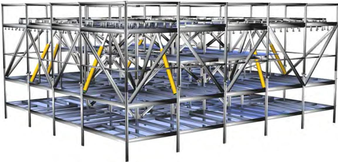
**Figure 6.** arrangement of dampers in 250 W 55th Street. Image copyright Arup.
