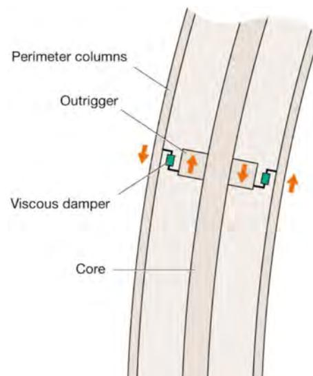
**Figure 1.** the damped outrigger concept (Image copyright Arup).
