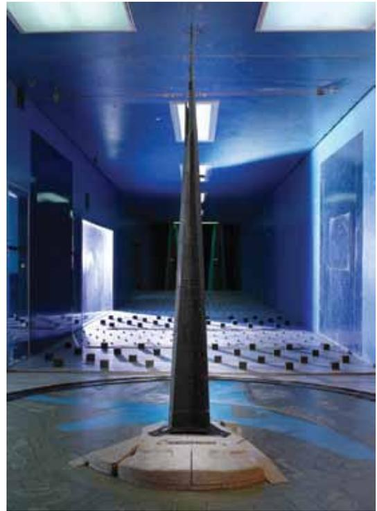
Figure 9. : Kingdom Tower wind tunnel testing. (Source: Jeddah Economic Company/ Thornton Tomasetti)
