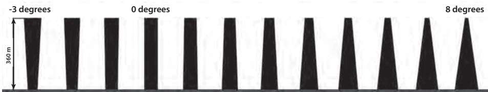
Figure 5. The variation of the angles of the tapering models.
