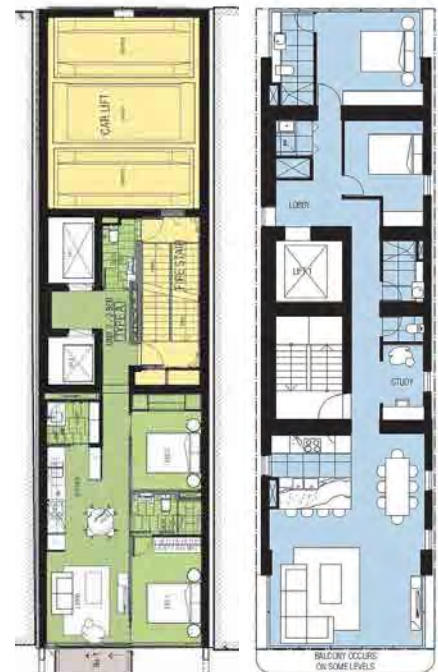
Figure 5. Typical plans showing the the automated car stacking at the rear of the building and the double-H structural configuration. © Fender Katsalidis Architects
