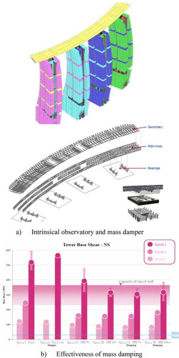
**Figure 1.** Intrinsic mass damping.
