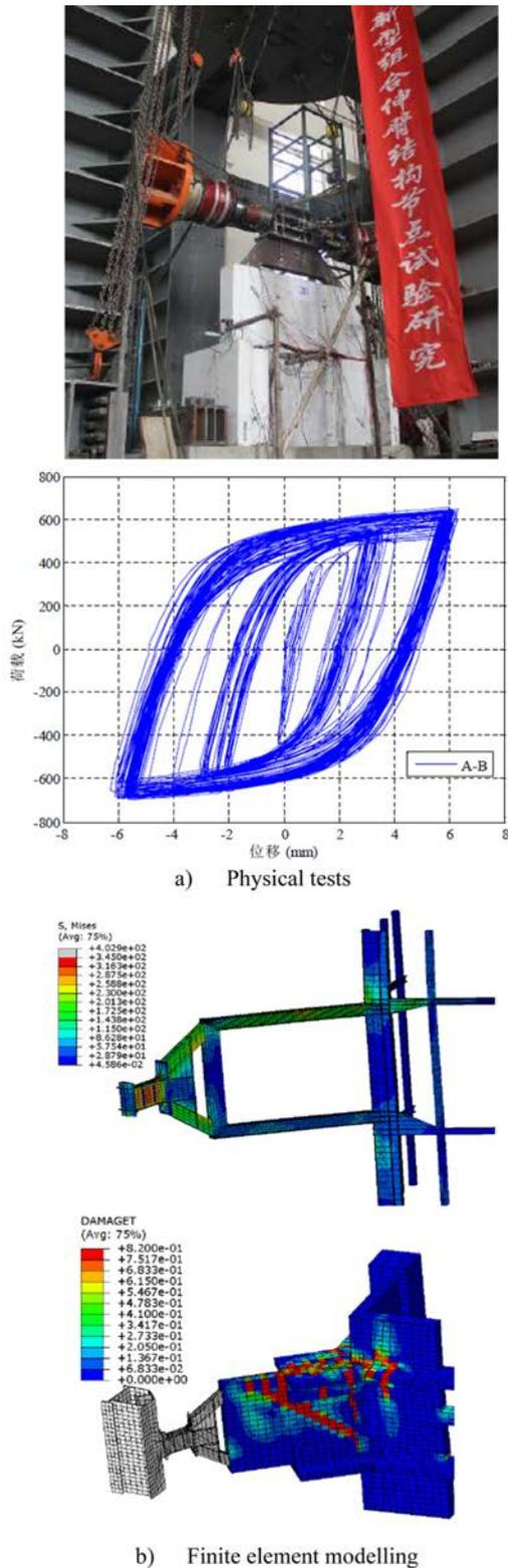
Figure 4. Study on hybrid outrigger.
