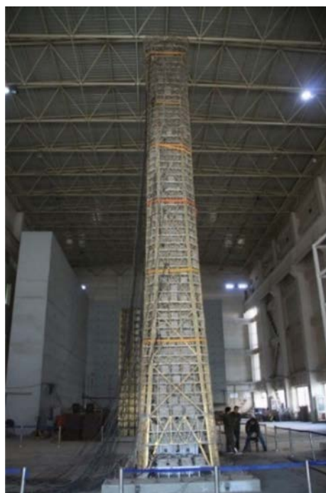
Figure 15. Shaking table test.
