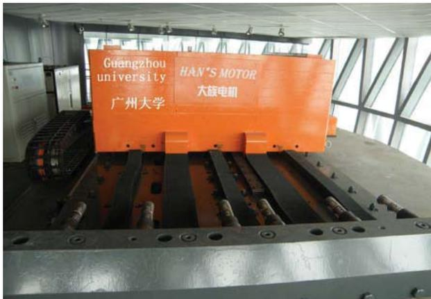
Figure 9. AMD driven by linear induction motors © EERTC
