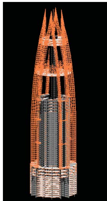
Figure 11. Finite Element Model of Spire and Crown
