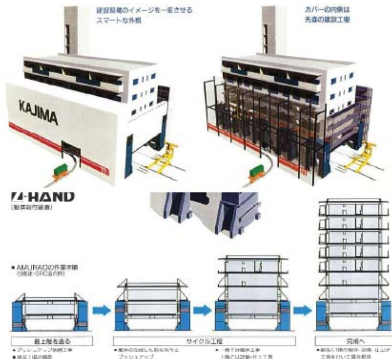
Figure 12. Automatic Up-Rising Construction by Advanced Technique (AMURAD)-method © Kajima
