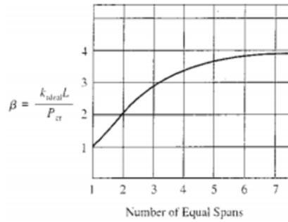
Figure 9.13.5 Variation of required spring constant for column with number of equal unbraced spans.
