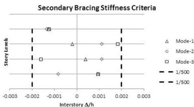
Figure 11. Lateral deflection of the diagrid structure under initial imperfection and P- $\Delta$  effect.
