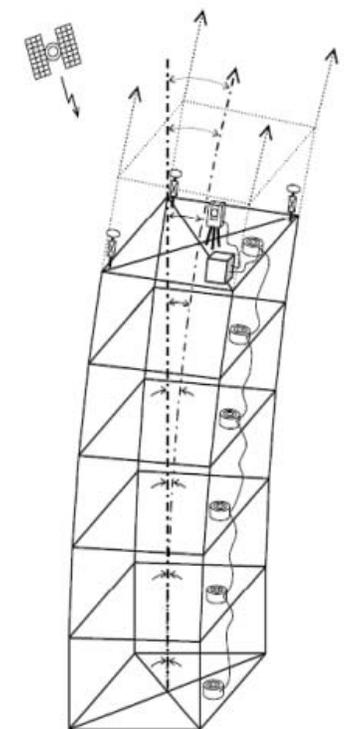
Figure 7. Schematic impression of the measurement of the lateral movement © Samsung C&T
