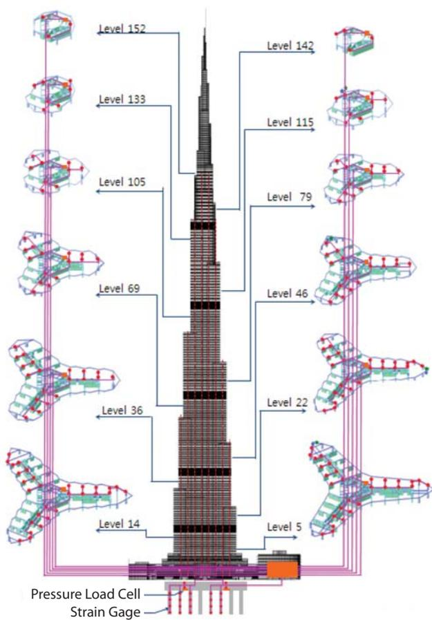
Figure 8. Strain Gage Monitoring System © Samsung C&T
