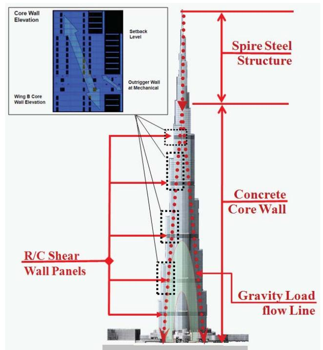
Figure 3. Lateral Load Resisting System © Samsung C&T
