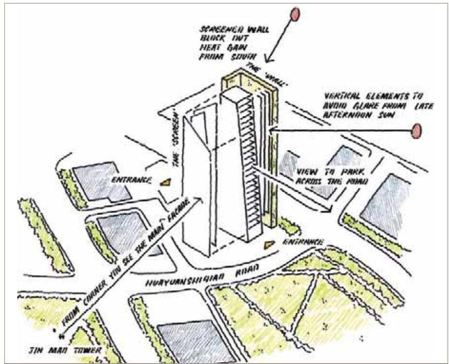
Figure 8. Different solar and amenity requirements governed the cladding design on each elevation of the BEA Tower in Shanghai (TFP Farrells)
