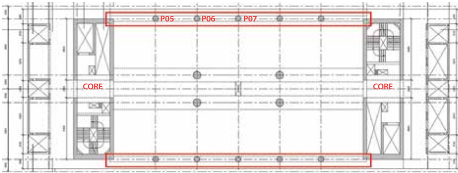
Figure 2. Typical floor plan. The red boxes show the location of the belt trusses at levels 23 and 49 only. The red text shows the location of elements whose vertical displacements were compared.
