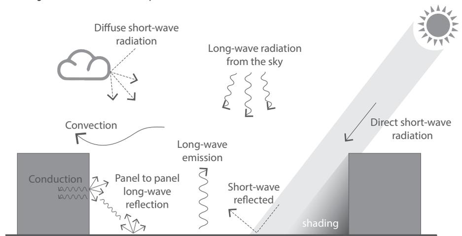
Figure 6. Overview of the full energy balance that needs to be calculated, for every hour of the year, for every data point within the urban domain.
