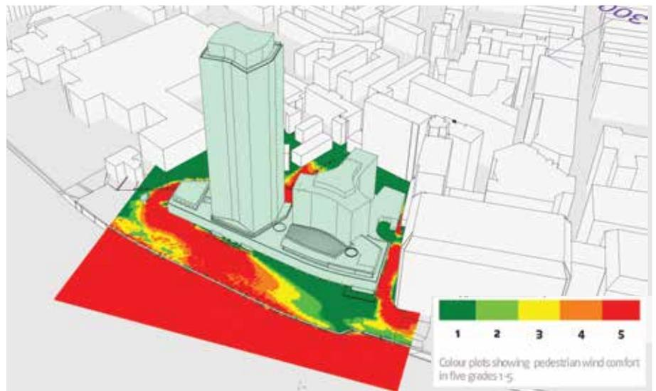
Figure 11. Year-round pedestrian wind comfort visualization on a horizontal plane at 1.5 m above grade, according to Dutch Wind Nuisance Criteria, for the Millbank Tower.
