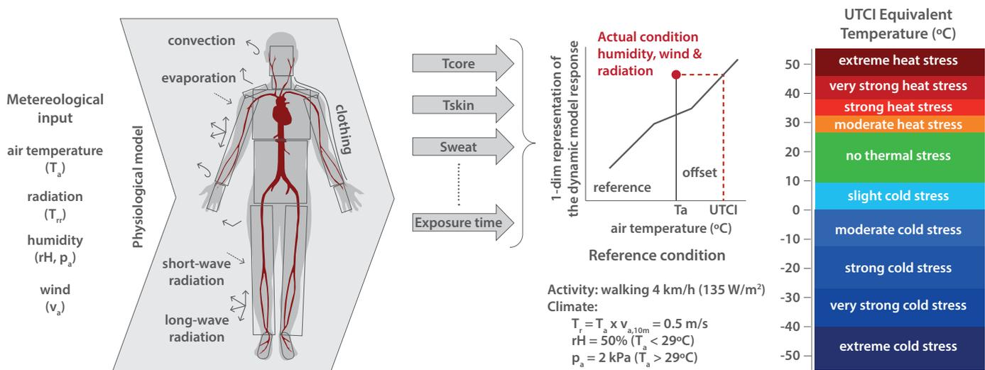
Figure 4. The Universal Thermal Comfort Index (UTCI) Equivalent Temperature identifies comfort in an urban space via a relative temperature scale.
