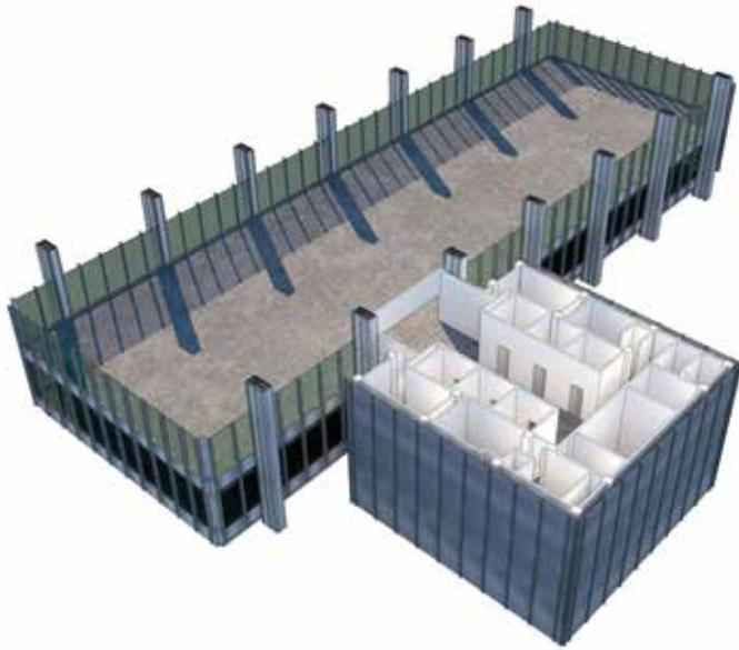
Figure 3. Inland Steel Building, Chicago (1957) – full floor plate reconstruction.
