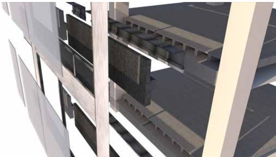
Figure 10. Equitable Building, Portland (1949) – cladding detail reconstruction, showing the location of perimeter air-conditioning cabinets.
