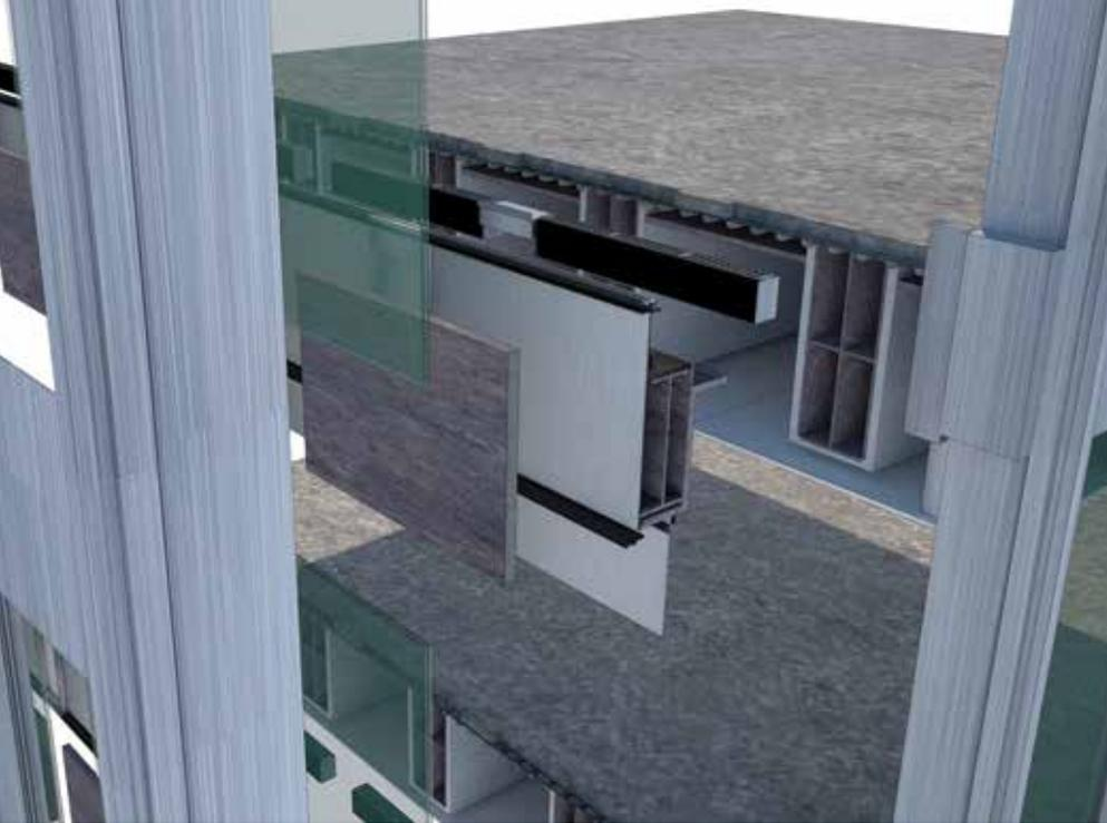
Figure 8. Inland Steel Building, Chicago (1957) – exploded cladding detail.
