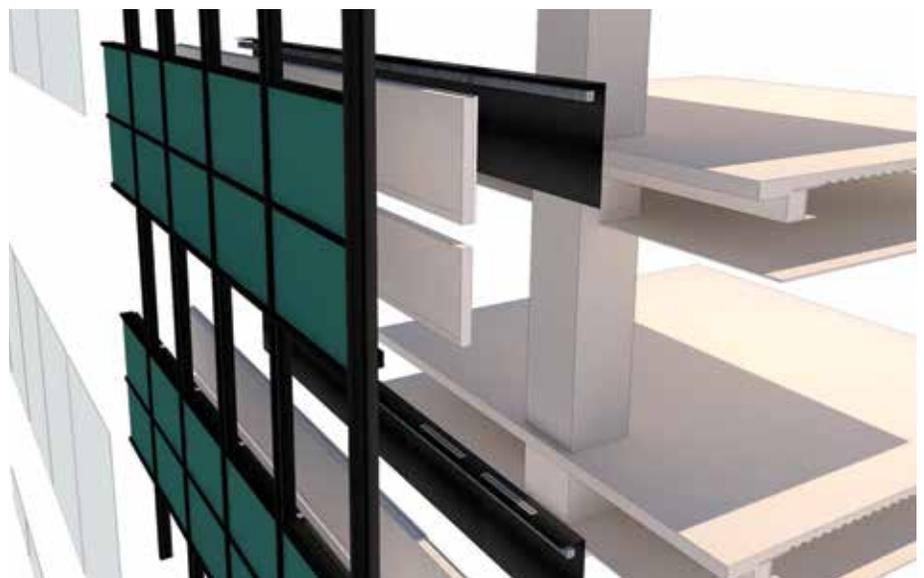
Figure 7. Lever House, New York (1953) – exploded cladding detail.
