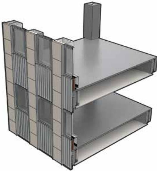
Figure 5. Prudential Building, Chicago (1954) – cladding detail reconstruction.
