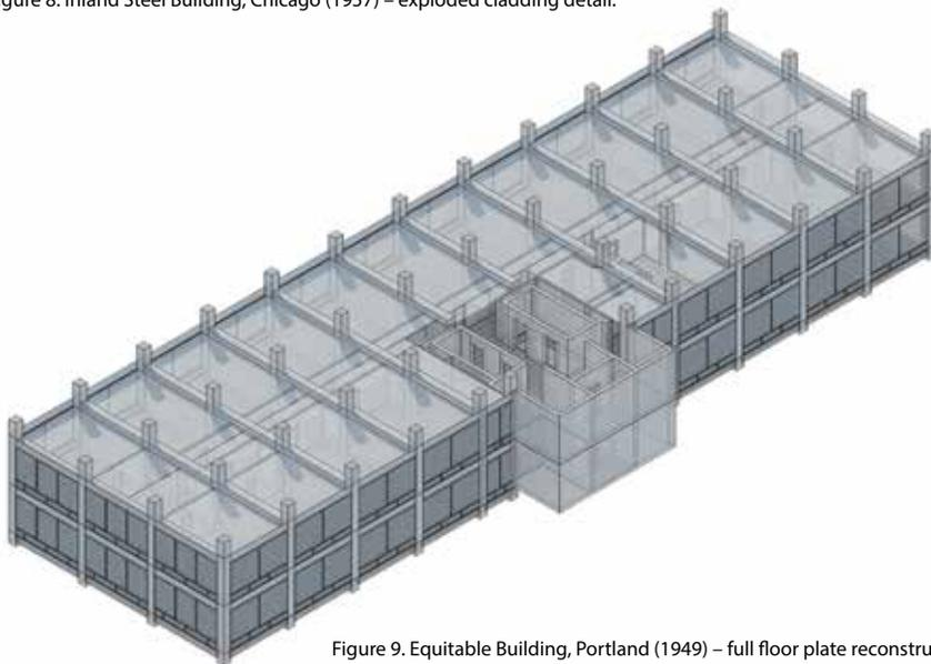
Figure 9. Equitable Building, Portland (1949) – full floor plate reconstruction.
