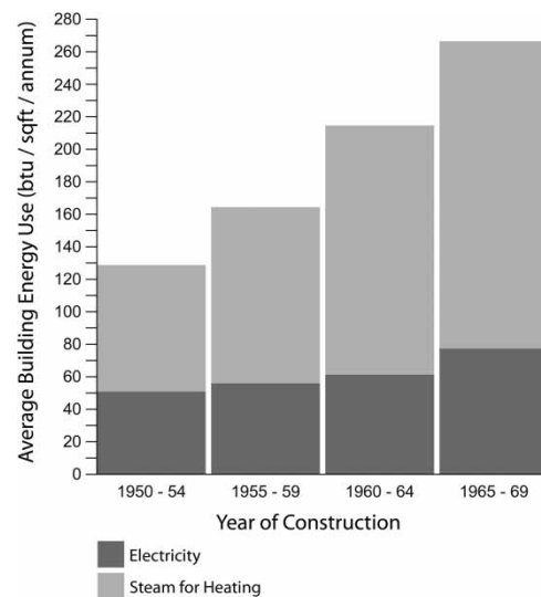
Figure 5. Average primary energy consumption of 86 office buildings constructed in Manhattan between 1950 and 1970. 30
