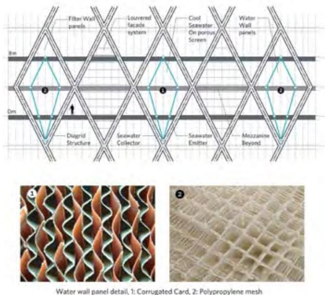
Water wall panel detail, 1: Corrugated Card, 2: Polypropylene mesh
