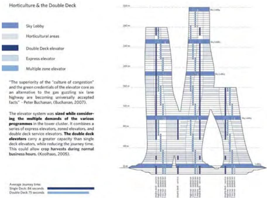
Figure 11. Double Deck Elevator - Tower Diagram
