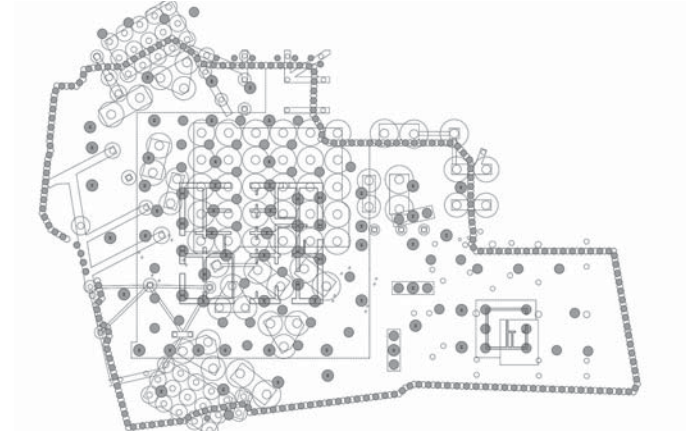
Figure 3. Existing and new piles at the Shard. © WSP
