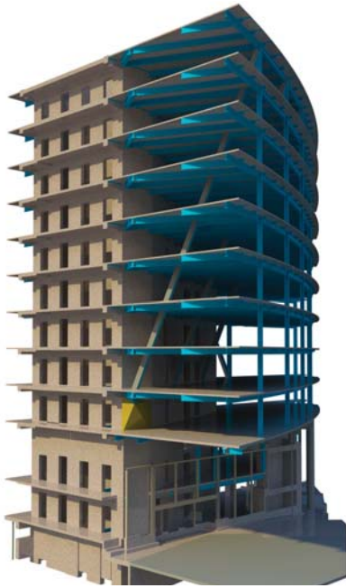
Figure 6. The Place – raking columns and corbel. © WSP
