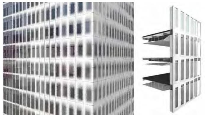
Figure 11. The facade concept was realized using a practical and efficient unitized curtain wall with ceramic frit variations. (Source: NBBJ)
