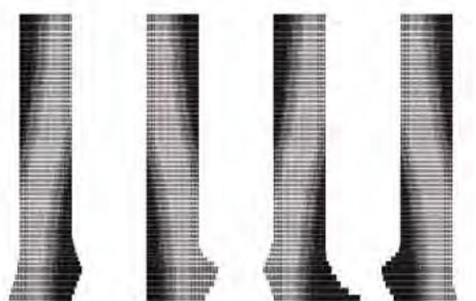
Figure 10. The elevations of the tower were developed using a parametric system which allowed the designer to integrate solar analysis values and explore gradient overlays. (Source: NBBJ)
