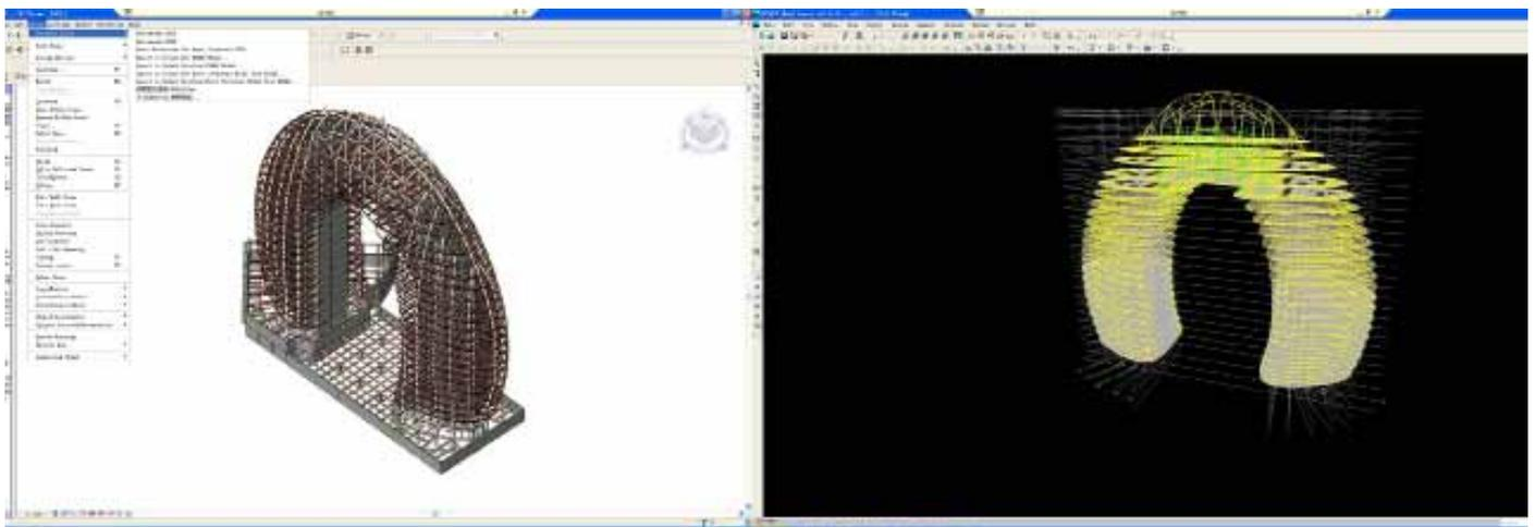
Figure 3. BIM model and structure analysis model two-way interaction
