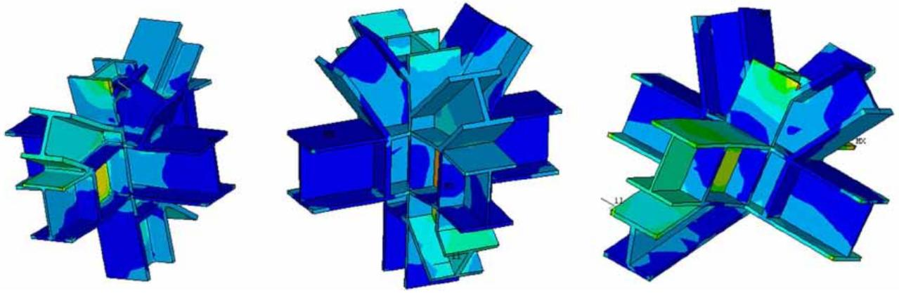
Figure 4. stress map of the detail connection
