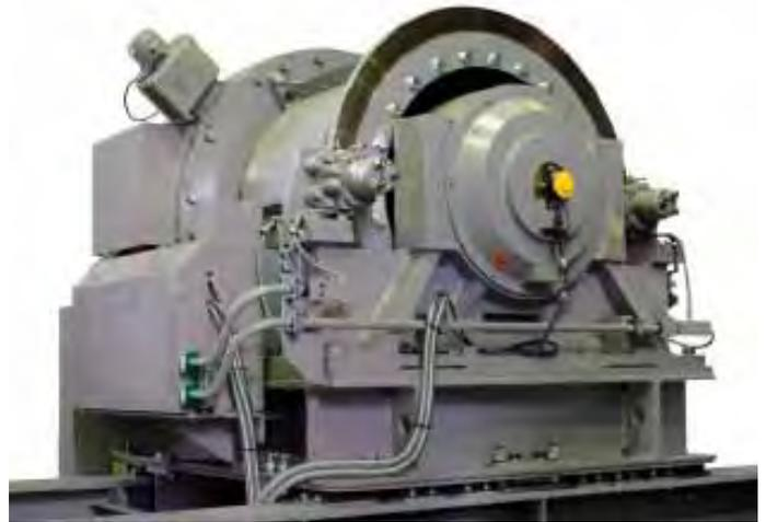
Figure 3. PM Traction Machine (Source: Mitsubishi Electric)
