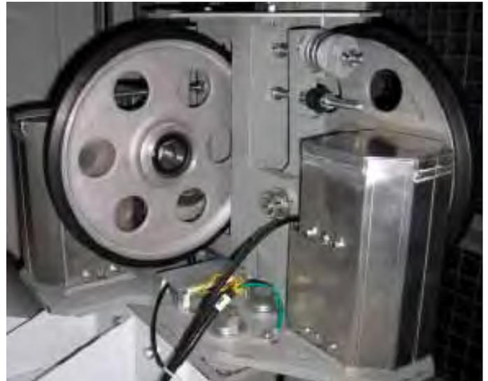
Figure 6. Active Roller Guide (Source: Mitsubishi Electric)
