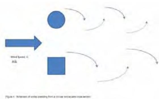
Figure 4. Schematic of vortex shedding from a circular and square section
