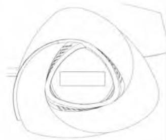
Figure 6. 'Rotating' cross sections of the Shanghai Center
