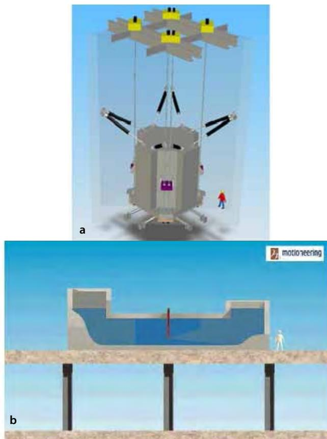
Figure 8. (a) Schematic of a simple pendulum Tuned Mass Damper (TMD), Schematic of a Tuned Liquid Column Damper (TLCD)
