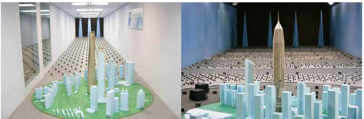
Figure 5. (a) Shanghai Center wind tunnel model, (b) Ping An Finance Center wind tunnel model
