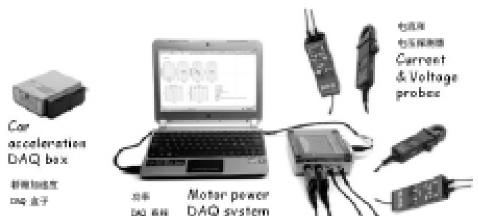
Figure 4. KONE ESiteSurvey™ measurement gear 图4. 通力电梯ESiteSurvey™ 测量工具
