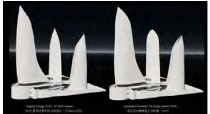
Figure 12. Baku Flame Towers – Optimization of tower shape to rationalize façade installation
