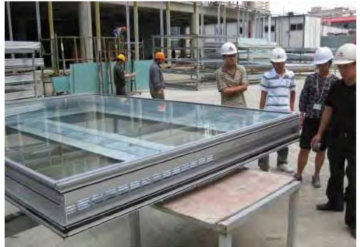
Figure 2. Siemens Center Shanghai – prefabricated large double skin façade units (Jiang-He CW contractor plant)
