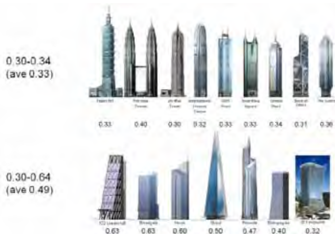
Figure 3. Asia vs London Wall: floor (Source: Davis Langdon) 图3. 亚洲vs. 伦敦：外墙-底台面积比率 (出自: Davis Langdon)
