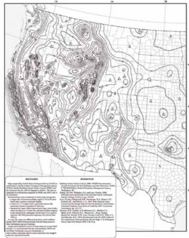
Figure 2. Seismic Design Criteria – Western U.S. (ASCE 7-10) (source: American Society of Civil Engineers)
