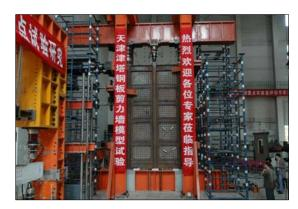
Figure 9. SPSW Assembly Test Set Up
