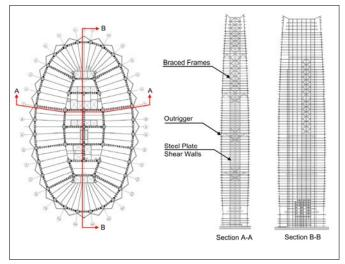
Figure 2. Typical Structural Plan, Sections
