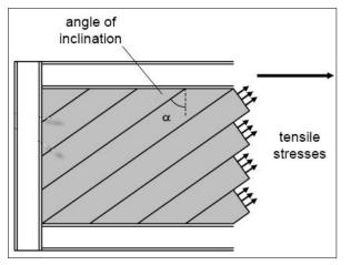
Figure 6. Tension Field Action Angle
