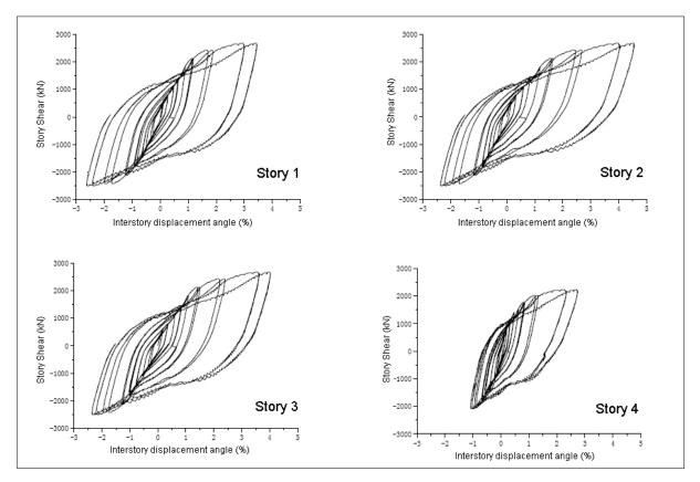
Figure 11. Story Shear vs Inter-Story Drift
