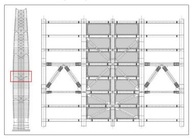
the tower core, around and service passenger elevators as well as stairways and mechanical rooms. The outrigger trusses, which are placed in the short direction of the tower plan, consist of structural steel bracing connecting the interior shear wall core with the perimeter moment-resisting ductile frame (Figure 3).
