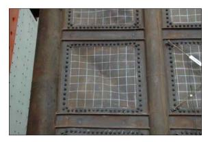
Figure 10. SPSW Panel after Test
