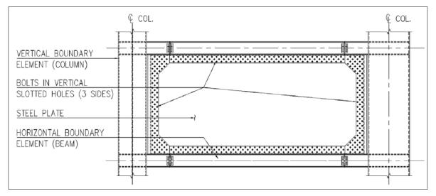
Figure 8. Typical SPSW Elevation
