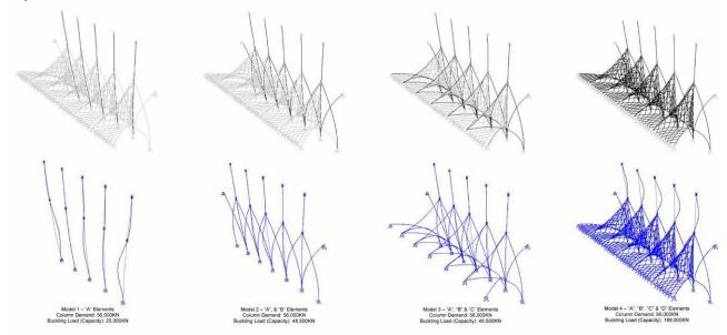
Fig. 5 Lamella Buckling Analysis Models
