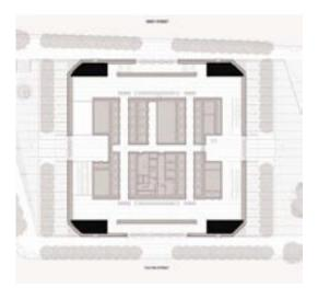
Figure 10: Freedom Tower - Ground Floor Plan with staircases shaded. (by author; used by permission of the cipyright holder)
