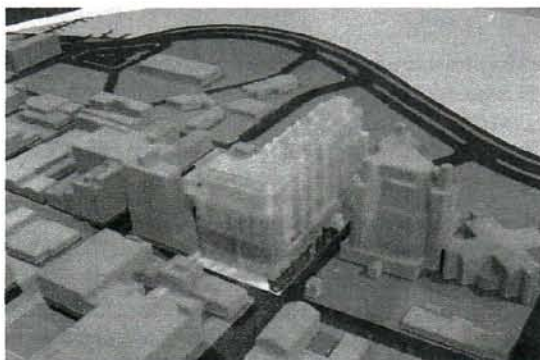
Figure 8: Simultaneous pressure data collection applied to a midrise condominium in Miami, Florida (510 taps).
