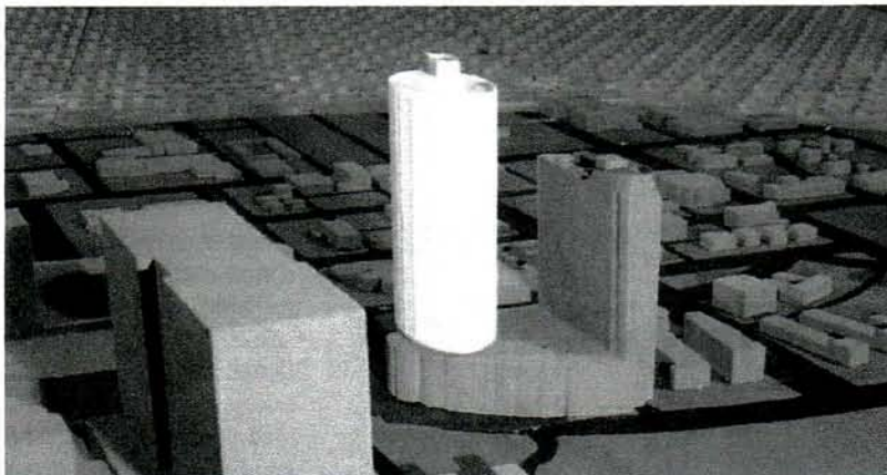
Figure 18: The oval building in the centre generated large torsional loads on the rectangular building to the right by partially shielding the dominant winds on its wide face. Fortunately it was tested with and without the oval building in place during a previous study and was designed to accommodate the torsional loads. How many buildings are not assessed in this manner?
