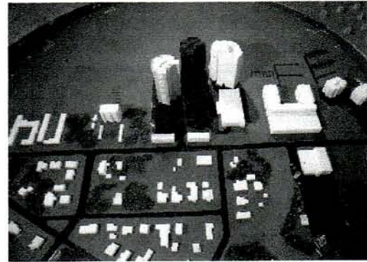
Figure 11: Thirty-storey Florida condominium, with tall proximate neighbours, used to compare balsawood force balance (shown here on the left as the twin building) data with the simultaneous pressure technique. The subject building is the middle one. Note that north is at the top of the photograph.
