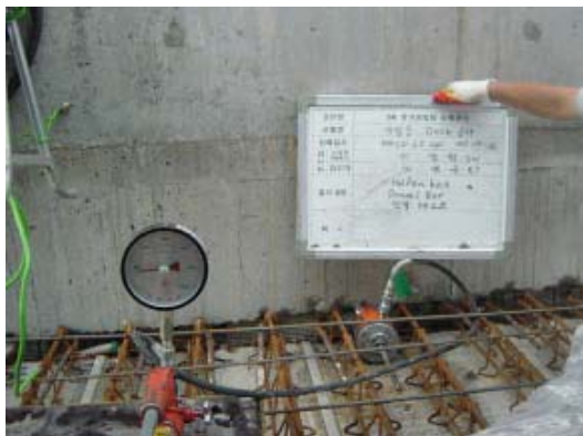
Fig. 18. Tension Test of Reinforcement Embedded in Halfen Box
