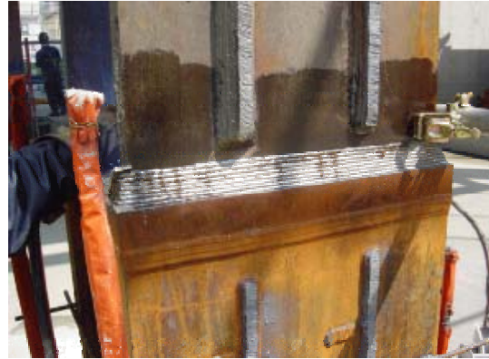
Fig. 10. Weld Size Examination of Column Connection
