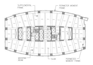
Figure 10 Typical Framing Plan.
