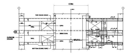
Figure 6 Outrigger Elevation.
