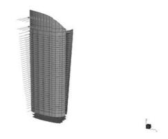
Figure 21 Westerly wind pressures apply to global FEM model.
