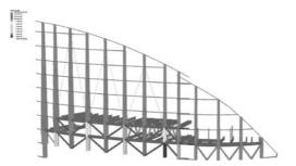
Figure 26 West sail finite element framing model.
