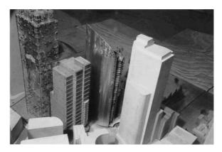
Figure 19 Aero-elastic model of Aurora tower.
