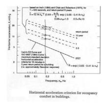
Figure 22 Building accelerations for occupancy comfort.
