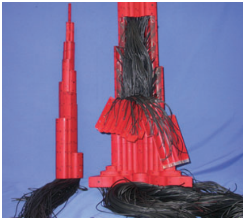
Figure 12. Detail of pressure taps in cladding pressure test model. (Image courtesy of RWDI)
