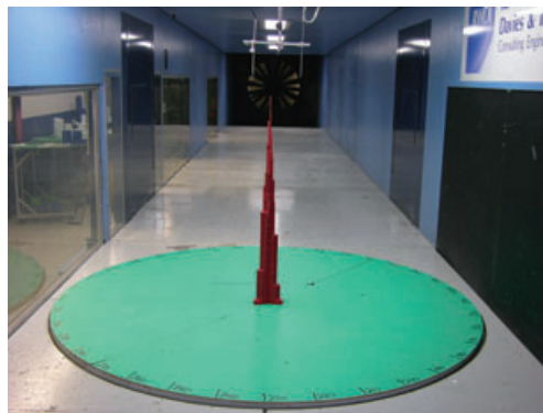
Figure 13. Cladding pressure test model at 1:500 scale, shown in wind tunnel. (Image courtesy of RWDI)
