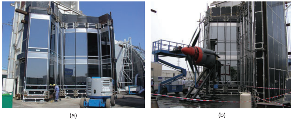
Figure 19. (a) Tower test mock-up assembly. (b) Tower test mock-up dynamic test for water penetration
